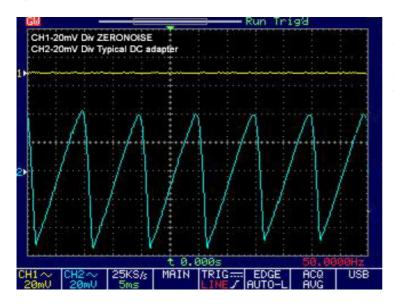
In the diagram (a) you can see the differences from a typical AC to DC adapter against **ZeroNoise Road**. The graphic shows that the DC output from the standard adapter introduces much more ripple noise into the signal as compared to the clean power produced by **ZeroNoise Road**.
