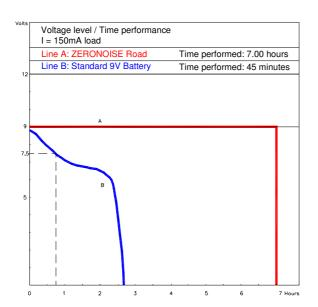
The above graph shows the huge difference in time of autonomy between a common 9V battery and the ZeroNoise Road power box: about 10 times more capacity and no degradation of output characteristics until the internal battery completely discharge.
