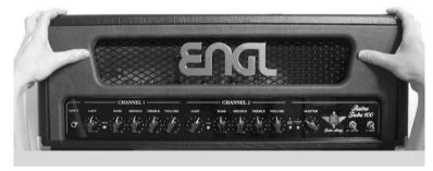
Fit the front panel frame into the front side deepening of the amp's housing;
