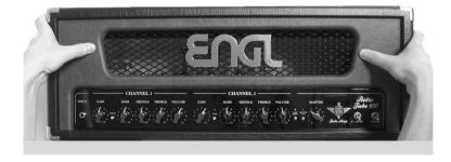
Push the front panel frame until the locking mechanism latches.
