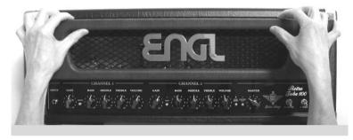
insert the bottom part of the front panel frame in the two milling grooves located at the base panel of the amp's housing;
