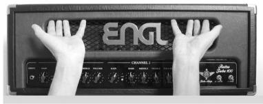
pull the front panel frame (without the grille!) until the locking mechanism unlatches;
